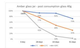
Figure 5 - Retinol recovery over 90 days under conditions of 5°C, 23°C and 40°C in amber glass jar packaging.
