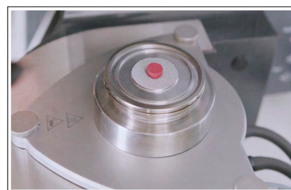
Figure 3. A lipstick sample on the serrated plate of the rheometer.
