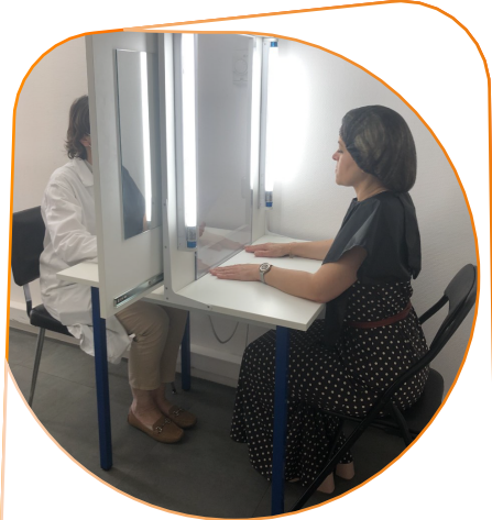
For the Face-to-Face assessment Subjects & Evaluators: An assessment table with standardized lighting using 3 neon lights (sides + top) is used. The volunteer is positioned with his or her abdomen pressed against the assessment table, arms laying on the table.
