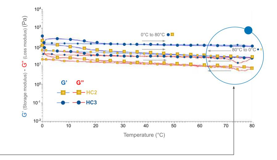
Due to fatty alcolhol removal, no sensitivity to temperature variations of HC2 and cold-processed HC3.
