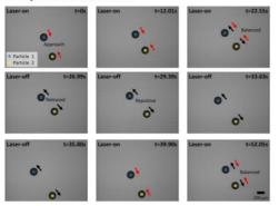
Microscopic images obtained during the migration of two particles upon laser-on and laser-off where the measured laser power was  $P_{dv} = 100 \text{ mW}$
